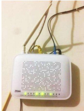
**Gambar 2. 12** Optical Network Unit (ONU)
