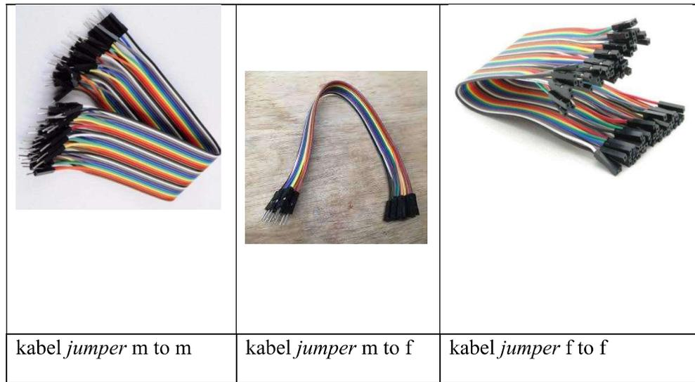
**Gambar 2. 17** Kabel *Jumper*
