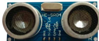
**Gambar 2.3** Sensor Ultrasonik
