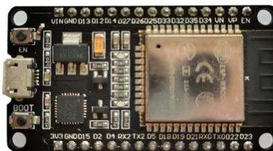
**Gambar 2. 5** Microcontroller ESP32
