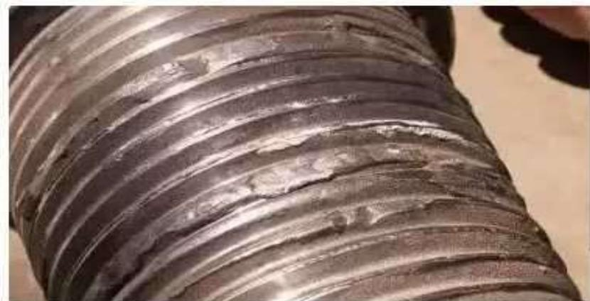
**Gambar 1.1** *Defect step thread*
