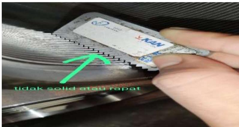
**Gambar 1.2** *Defect chatter thread*
