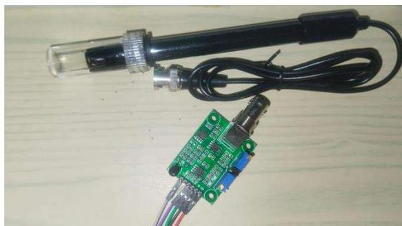
**Gambar 2.5** Sensor PH-4502C
