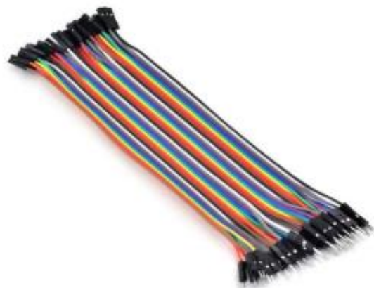
Gambar 2. 9 Kabel Jumper Sumber: (Santoso et al., 2021)
