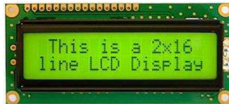
Gambar 2. 5 LCD 2x16 Sumber: (Suryantoro 2019)
