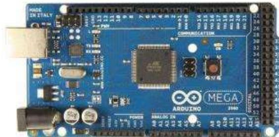
**Gambar 2. 2** Arduino Mega
