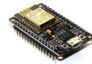
**Gambar 2.3** NodeMCU
