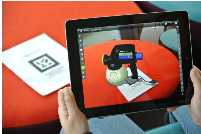
Gambar 2. 1 Contoh Augmented Reality using Marker Based Tracking
