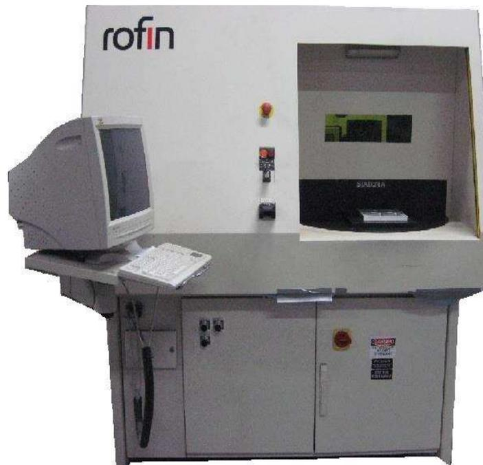
**Gambar 2. 3** Mesin Laser *Marking*
