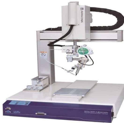
**Gambar 2. 4** Robot Soldering
