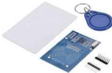
**Gambar 2. 4** Card Dan Sensor RFID MRC522
