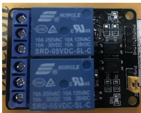
**Gambar 2.13** Relay 2 Channel
