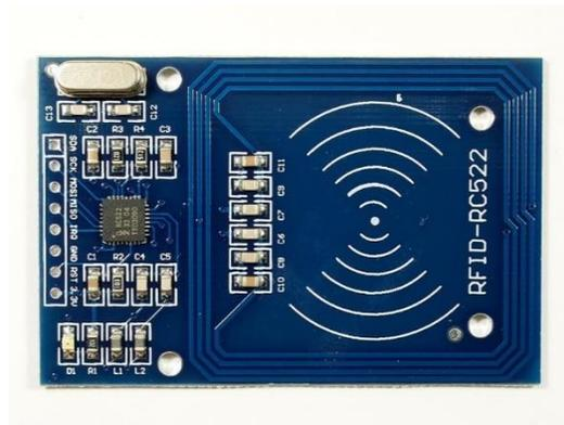
**Gambar 2.5** *Radio Frequency Identification (rfid)*
