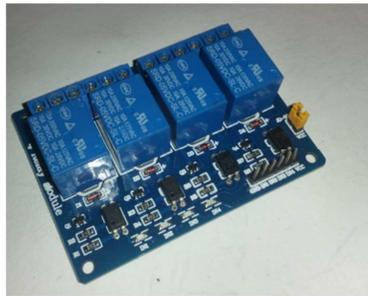
**Gambar 2.2** Relay 4 Channel
