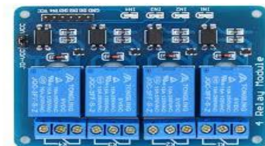
Gambar 2,5 Module Relay 4 Channel Sumber: Data Penelitian (2018)
