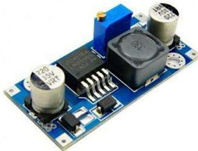
**Gambar 2.18** Module Converter Step Down Power Supply
