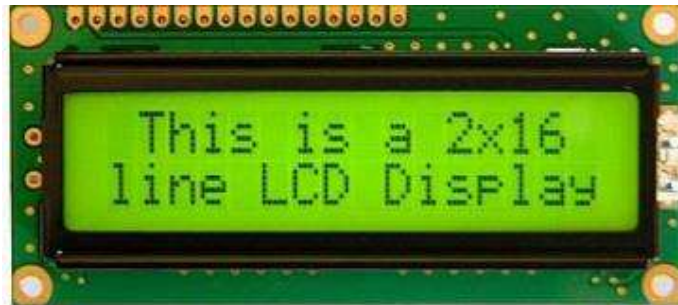
Gambar 2. 6. LCD 16x2 Sumber : (Rahman & Nawawi, 2017)
