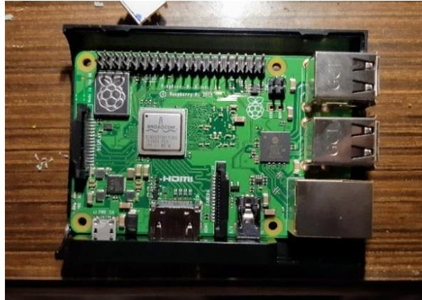
**Gambar 2.9** *Raspberry Pi 3 Model B+*
