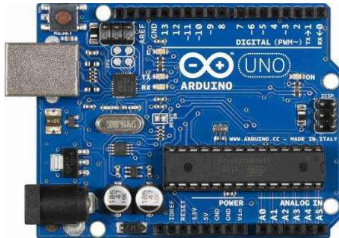
Gambar 2.2 Board Arduino Uno Sumber: (Afdali, Daud, & Putri, 2017)
