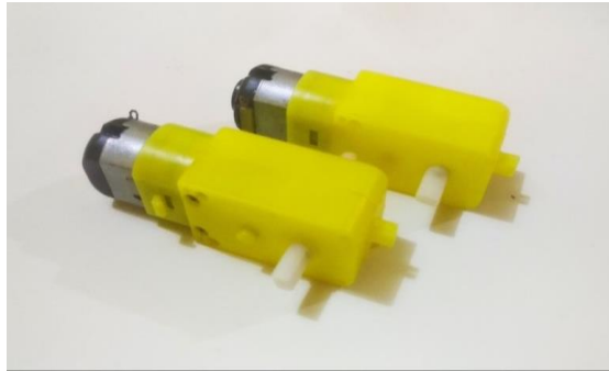
Gambar 2.5 Motor DC Direct Current Sumber: (Penelitian, 2020)
