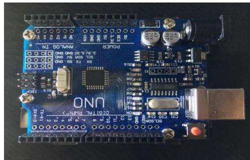
**Gambar 2.2** Board Arduino Uno
