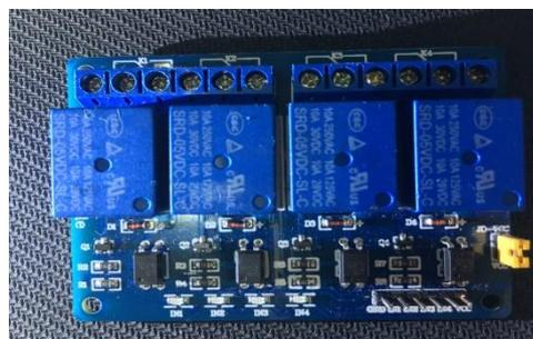
**Gambar 2.4** Relay module 4 channel 5volt
