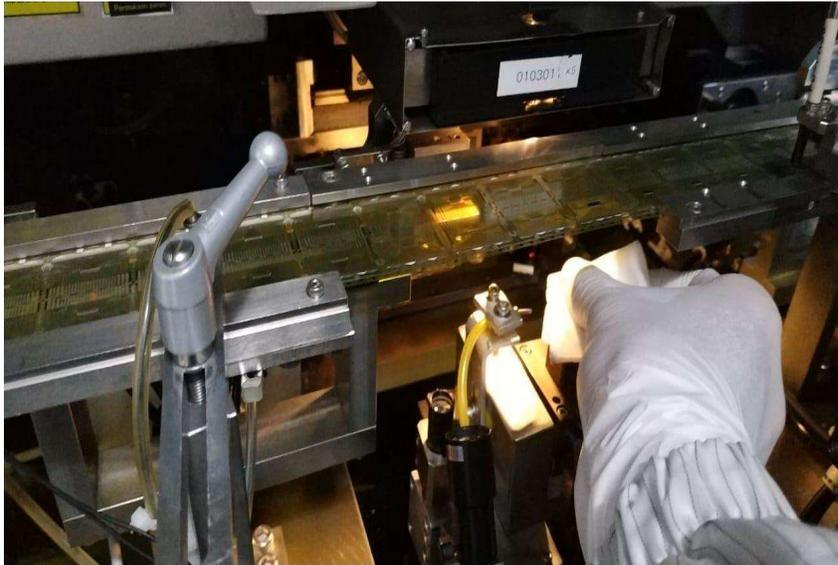
**Gambar 2.9** Membersihkan Bonding Stage
