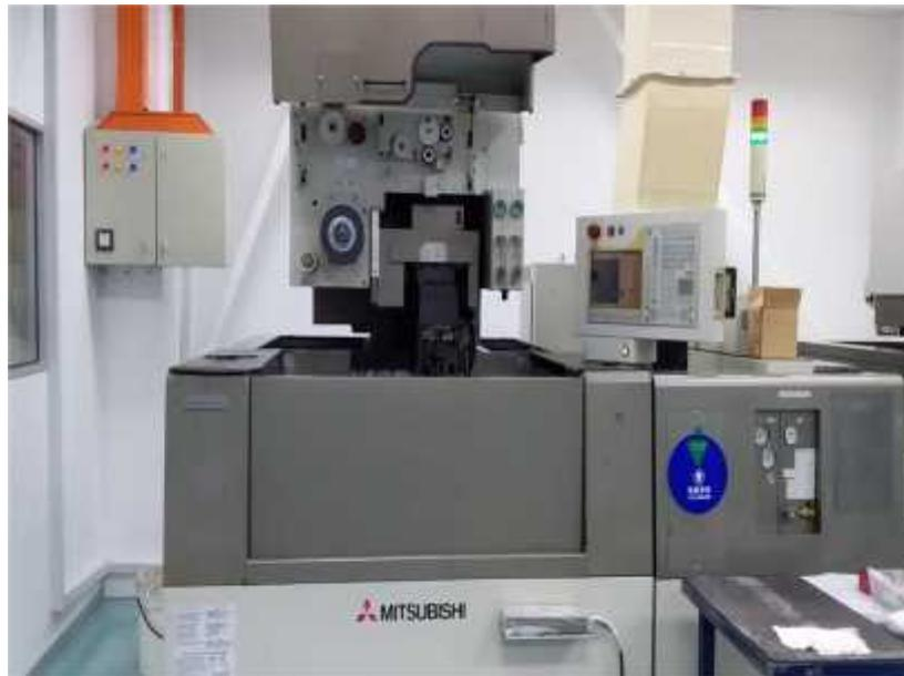
**Gambar 2.4** Mesin *CNC WIRE CUT*
