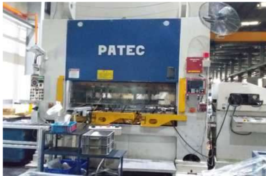
Gambar 2.1 Mesin Stamping Auto (Sumber: PT Amtek Engineering Batam, 2018)
