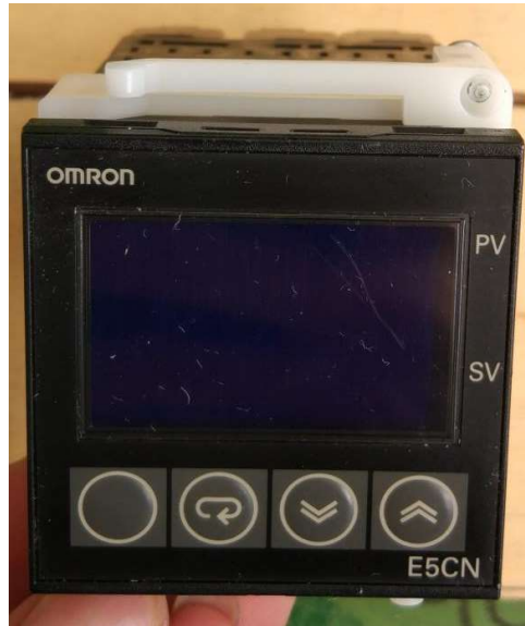
Gambar 13. Thermocouple temperature display
