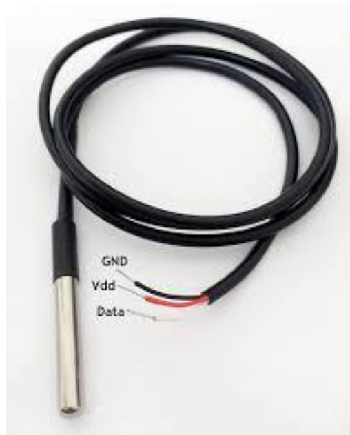
Gambar 2.2 Sensor DS18B20 Sumber: Data Penelitian (Alif et al., 2016)
