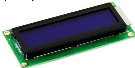
**Gambar 2.8** LCD 12X2
