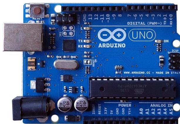
**Gambar 2.1** Microcontroller Arduino UNO
