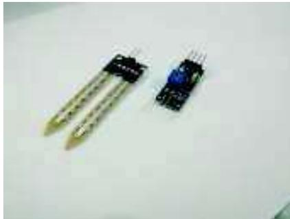
**Gambar 2. 2** *Soil Moisture Sensor*
