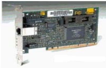
Gambar 2. 11 NIC (Network Interface Card) (Sari et al., 2013)
