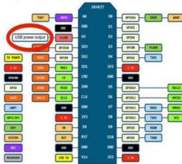
Gambar 2.2 Mapping PIN NodeMCU V3 Sumber: (Sahru & Rosa, 2017)
