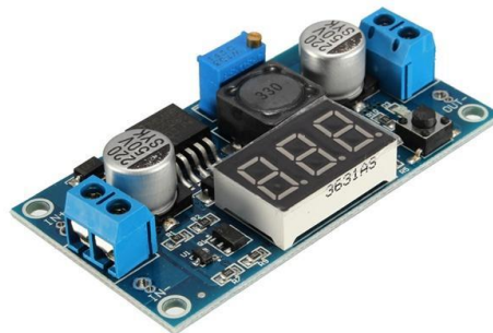
Gambar 2. 13 Regulator Stepdown DC-DC
