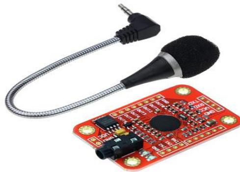
**Gambar 2.2** *Sensor Recognition Voice Module V3*
