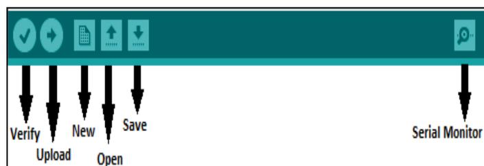
**Gambar 2.6** *Toolbar* IDE Arduino
