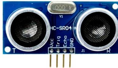
**Gambar 2.4 Sensor Ultrasonik**
