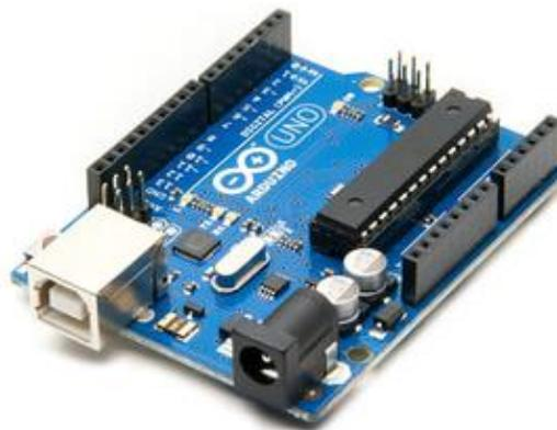
**Gambar 3. 3** Arduino UNO *Board* ATmega 328
