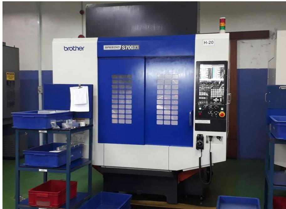
**Gambar 2.1** Mesin *CNC Milling*
