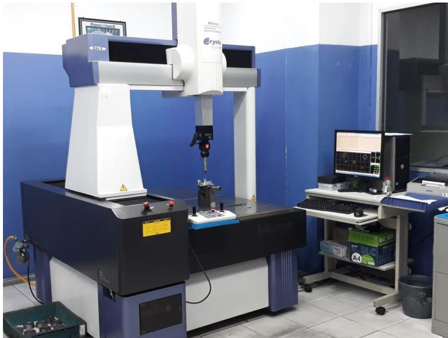
**Gambar 2.2** Mesin *Coordinate Measuring Machine*
