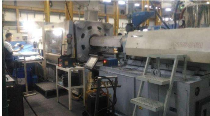
**Gambar 2. 1** Mesin *injection molding*
