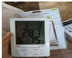
**Gambar 2. 2** Terometer Digital
