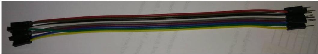
**Gambar 2.8** Kabel *jumper male to female*
