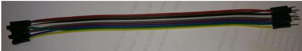
**Gambar 2.8** Kabel *jumper male to female*
