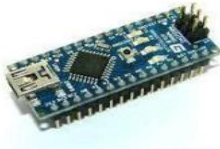
**Gambar 2.1,** Papan Arduino Nano.
