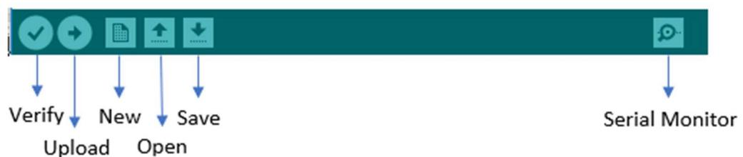
**Gambar 2. 4** Tampilan *Toolbar* IDE Arduino 1.8.5
