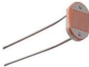
**Gambar 2. 2** LDR (*Light Dependent Resistor*)
