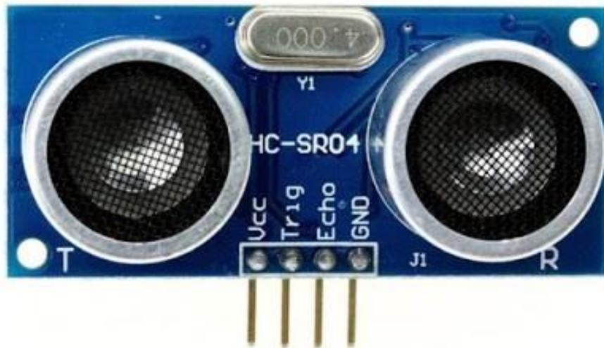
**Gambar 3.6 :** Sensor Ultrasonik
