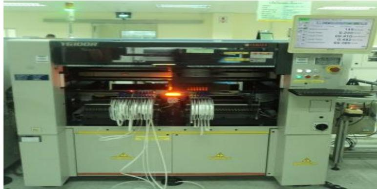
**Gambar 2.5** Mesin Pick up and Place
