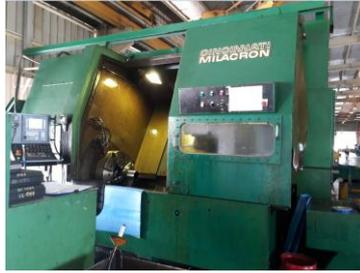
**Gambar 2.1** Mesin Bubut CNC
