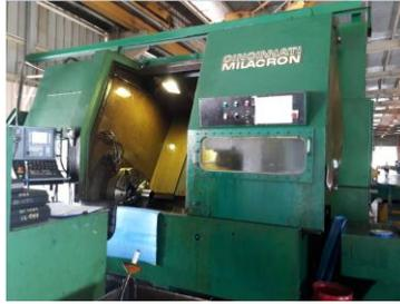
**Gambar 2.1** Mesin Bubut CNC
