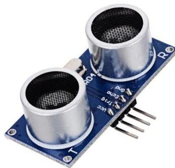
**Gambar 2.1** Sensor Ultrasonik
