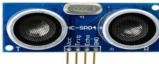
**Gambar 2.30** Sensor *Ultrasonik*
