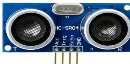
**Gambar 3.10.** Sensor *Ultrasonic*
