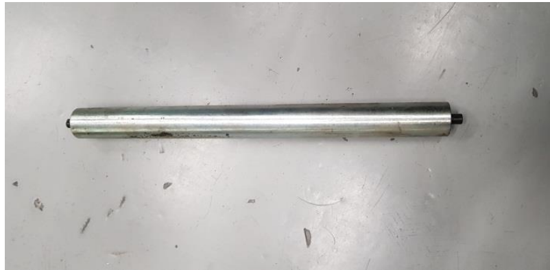
Gambar 2. 1 Support roller (material stanless)
