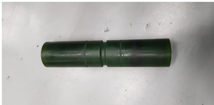
Gambar 2. 2 Drive roller (material PU)
