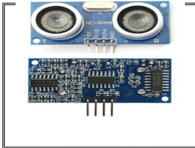
Gambar 2.5 Sensor Ultrasonic HC-SR04
